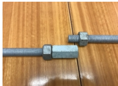
Figure 5. Bracing rods unscrewed from coupler (HERA, 2017)
