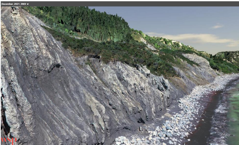
Figure 7: Lower section of Johnsons Hill landslide on Cape Palliser Road, UAV 3D model snip, with coastal erosion acting as a key contributor to slope instability. Model allows viewing of difficult-to-reach features.
