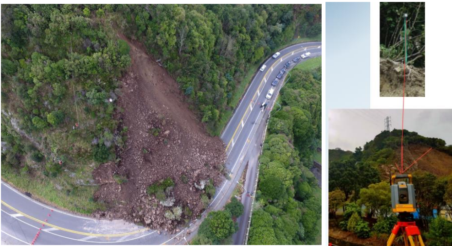
Figure 1: Ngaio Gorge Road, July 2017 rockslide and EDM target monitoring setup during earthworks
