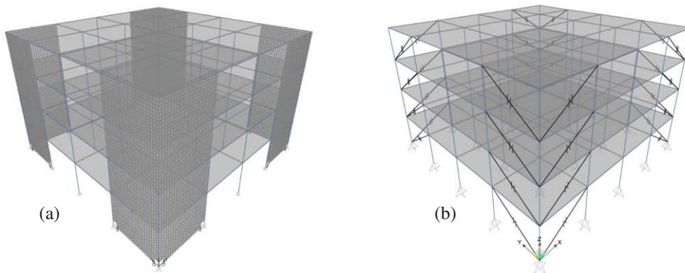
**Fig. 2** Numerical models: (a) rocking wall option (b) braced-frame option
