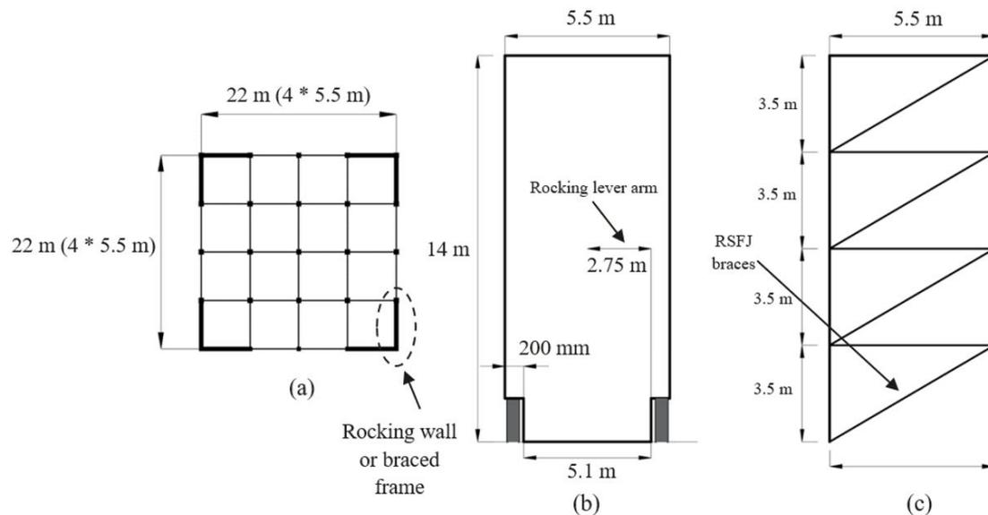
**Fig. 1** General configuration of the case study structure: (a) plan view (b) rocking wall option (c) braced frame option
