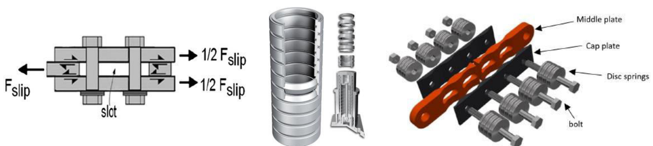
Figure 1: Low damage friction energy dissipators: (a) slip-friction joint; (b) friction rings springs; (c) resilient slip friction joint
