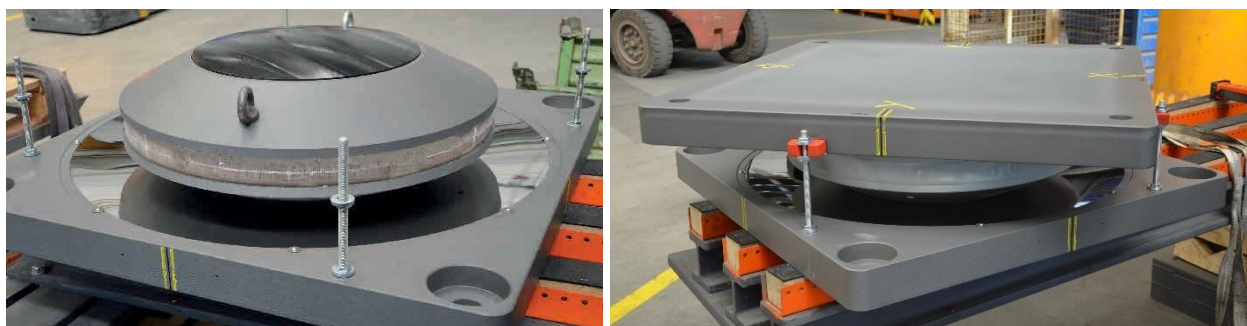
Figure 3: Open prototype without upper sliding plate (left) with conical inner puck with white Sylodyn ® pad inside and slider lens in black made of MSM ® ; assembled full device (right)
