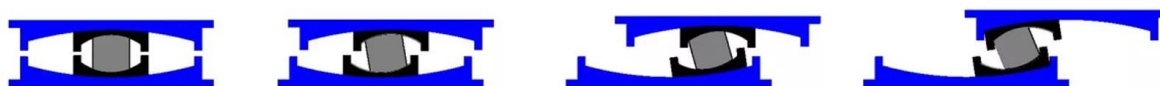
Figure 3.2: Schematic Showing Horizontal Displacement of Triple Pendulum Slider (courtesy Earthquake Protection Systems Ltd.)
