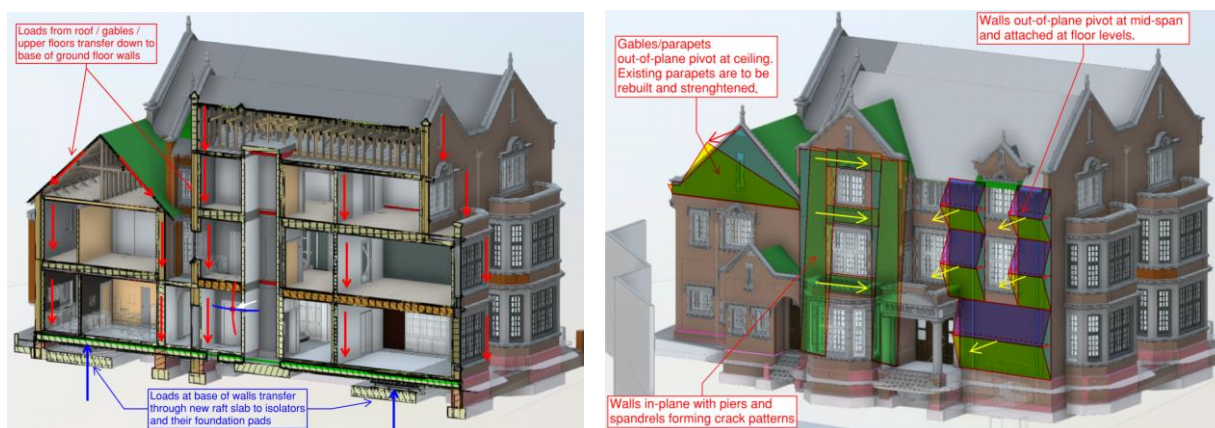
Figure 3.1: Overview of the Existing Structure and URM Walls.
